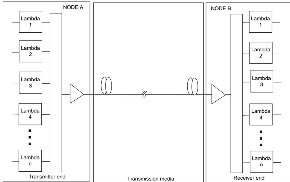
**Fig. 4 - Scenario 3 Post and pre-amplification**
