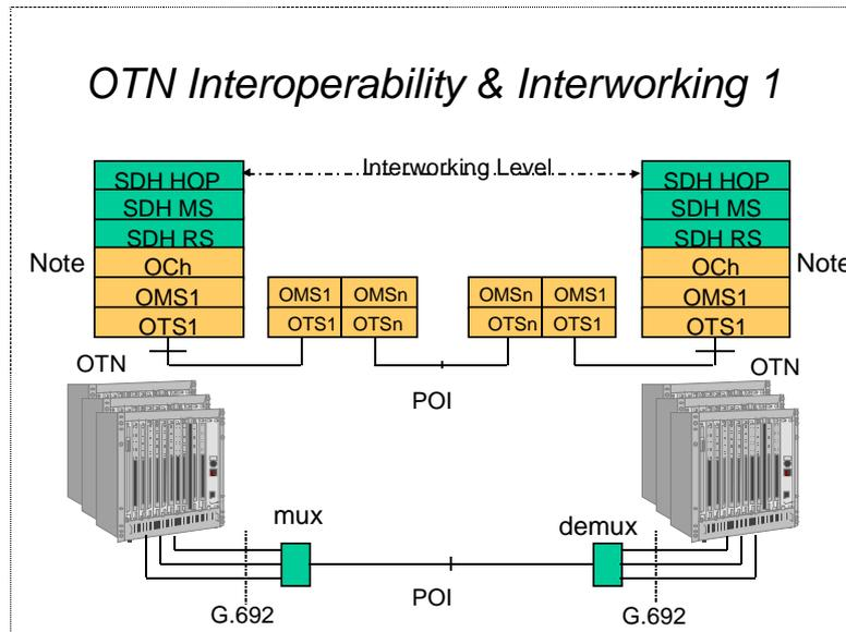
**Fig. 11 - Interoperability via passive multiplexers and demultiplexers**
