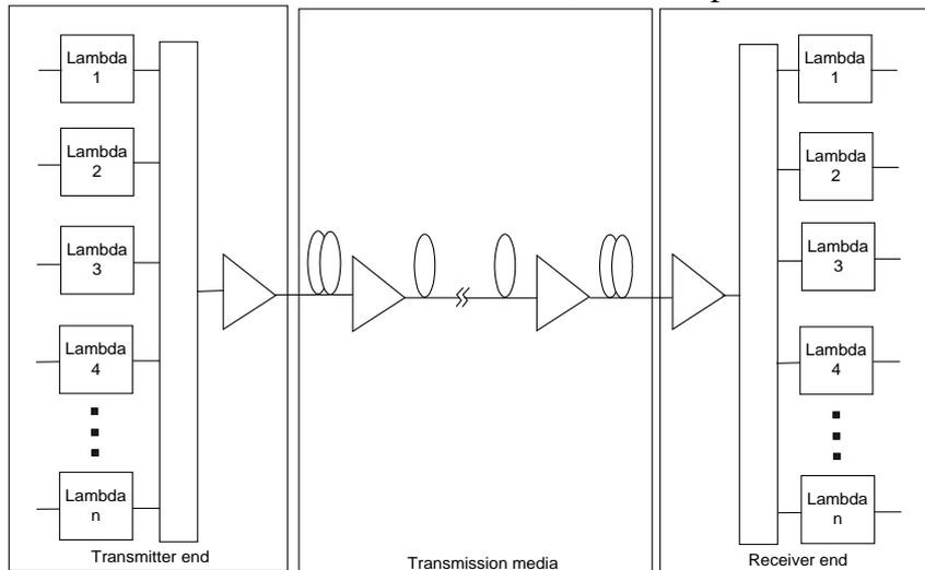
**Fig.1 - Functional elements of a WDM link**
