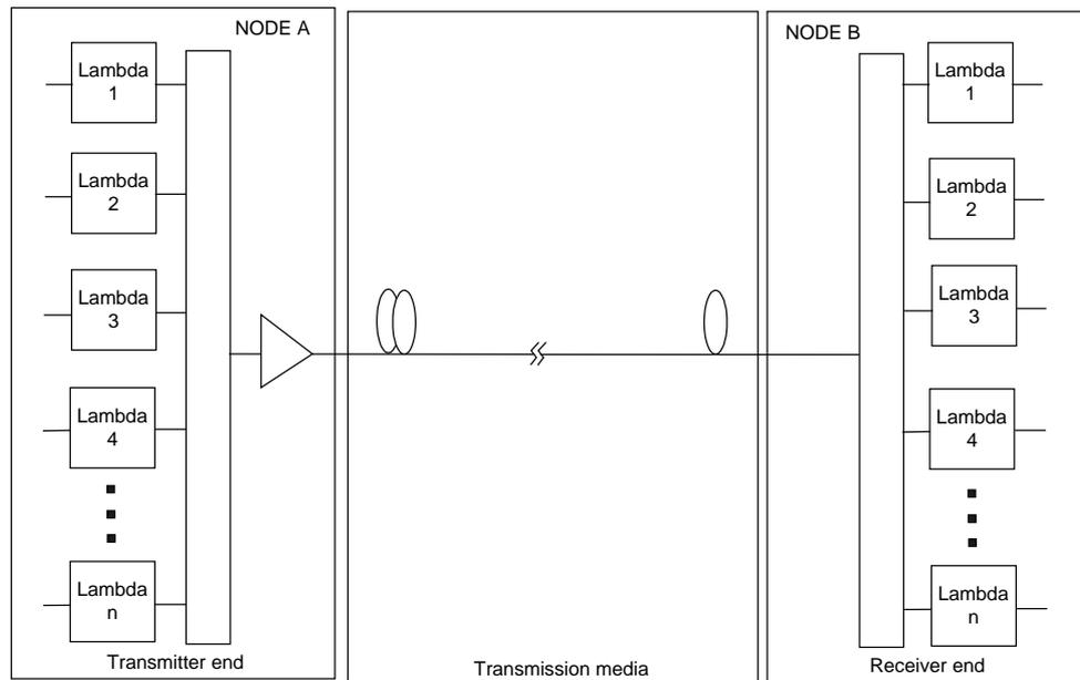
Fig. 3 - Scenario 2 Post amplifier at source
