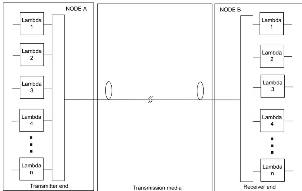
**Fig. 2 - Scenario 1 Unamplified short haul span**
