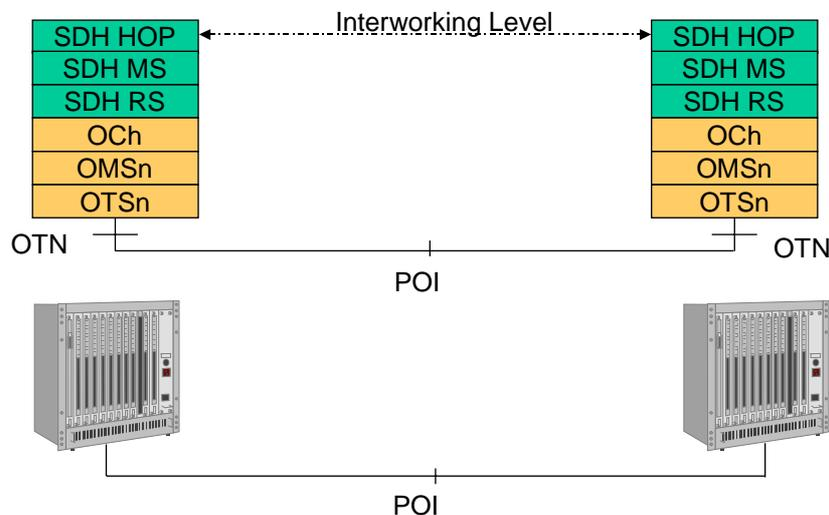
**Fig. 13 - Interoperability via a single box solution**
