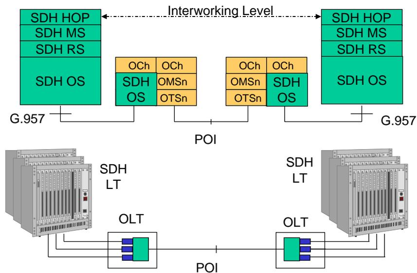
Fig. 12 - Interoperability using transponders
