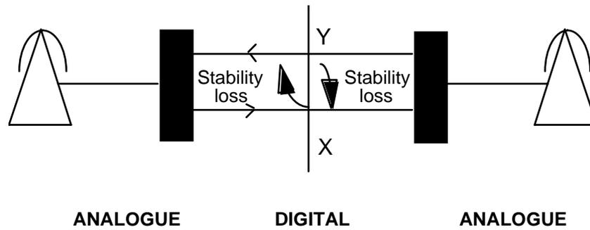
**Stability loss (X-Y and Y-X)  $\geq$  6dB**
