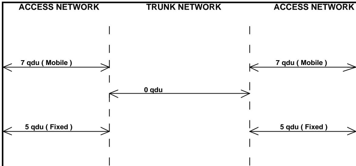
**Figure 11.1:** Reference model qdu limits
