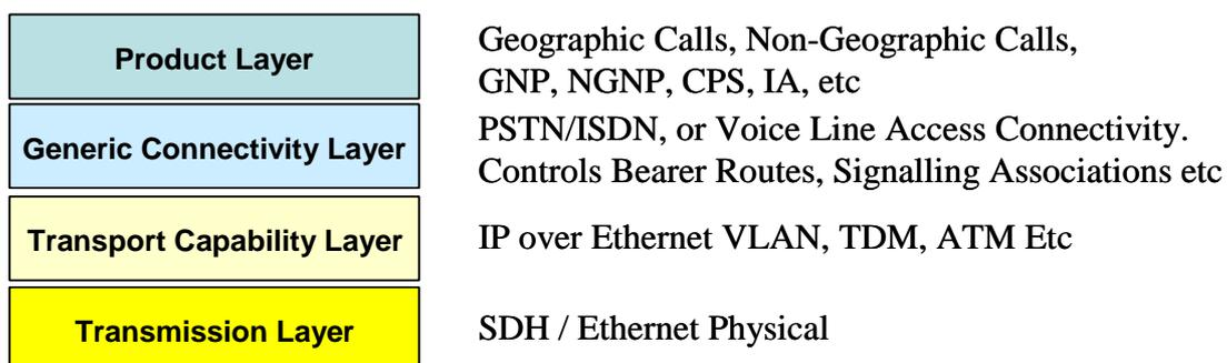
**Figure 1:-** Layering of functions for PSTN over a Multi-service Interconnect
