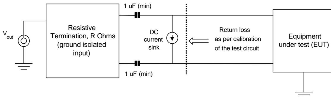
**Figure B.3 - PSD measurement set-up**
