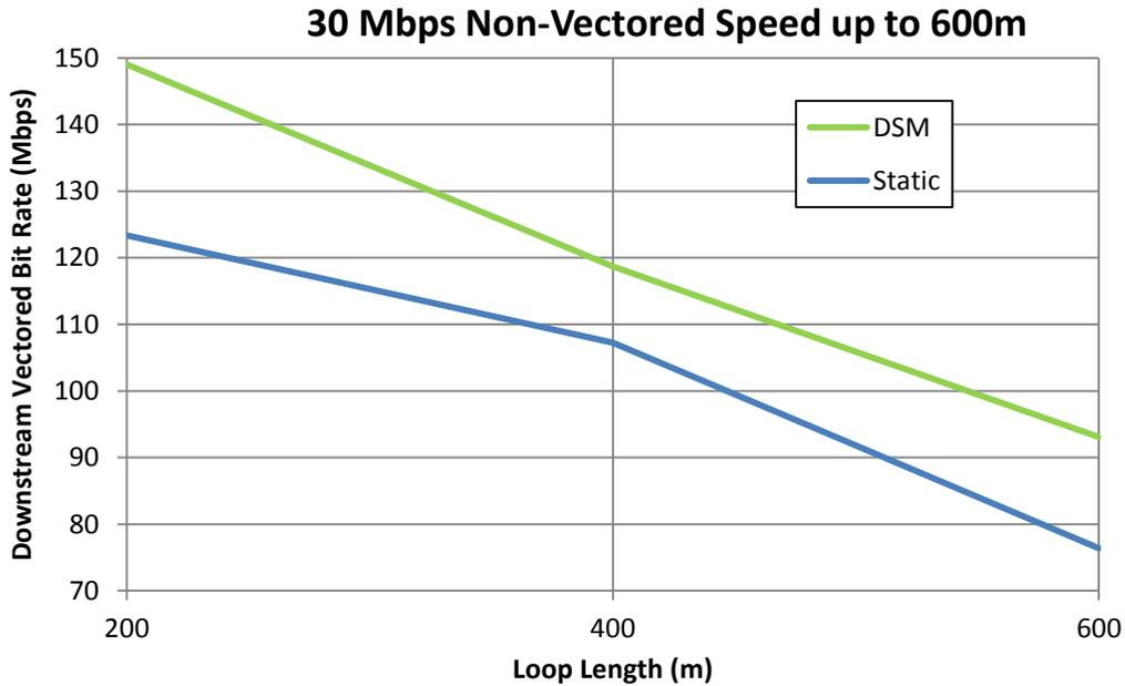
Figure 5. 1% worst-case vectored speeds with SSM ensuring 30 Mbps on non-vectorred lines no longer than 600 m. A 7 MHz SSM limit on non-vectorred lines ensures that they can transmit at least 30 Mbps on lines no longer than 600m.
