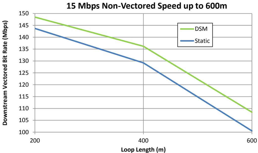
Figure 4. 1% worst-case vectored speeds with SSM ensuring 15 Mbps on non-vectored lines no longer than 600 m. A 2 MHz SSM limit on non-vectored lines ensures that they can transmit at least 15 Mbps on lines no longer than 600m.
