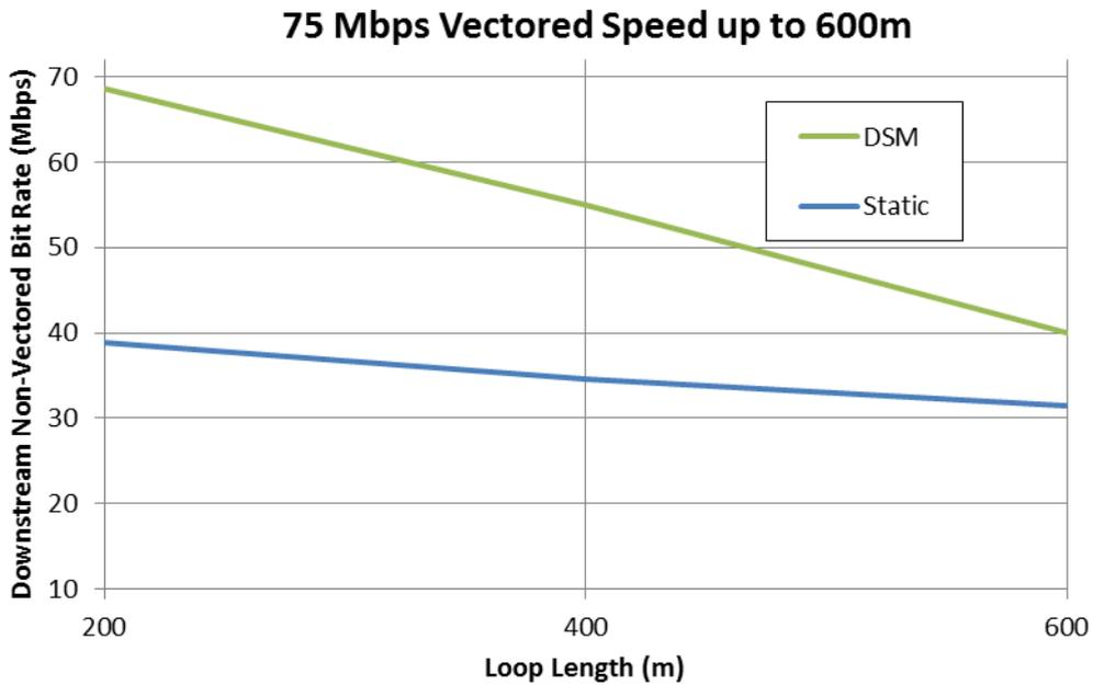
Figure 2. 1% worst-case non-vectored speeds with SSM ensuring 75 Mbps on vectored lines no longer than 600 m. A 7 MHz SSM limit on non-vectored lines ensures 75 Mbps on vectored lines no longer than 600m.
