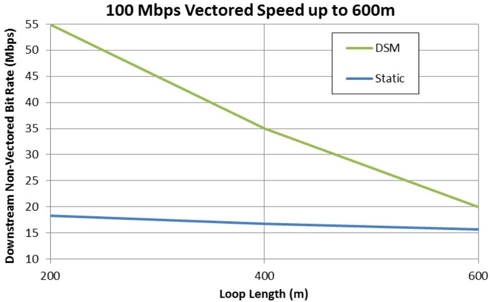
Figure 1. 1% worst-case non-vectored speeds with SSM ensuring 100 Mbps on vectored lines no longer than 600 m. A 2 MHz SSM limit on non-vectored lines ensures 100 Mbps on vectored lines no longer than 600m.
