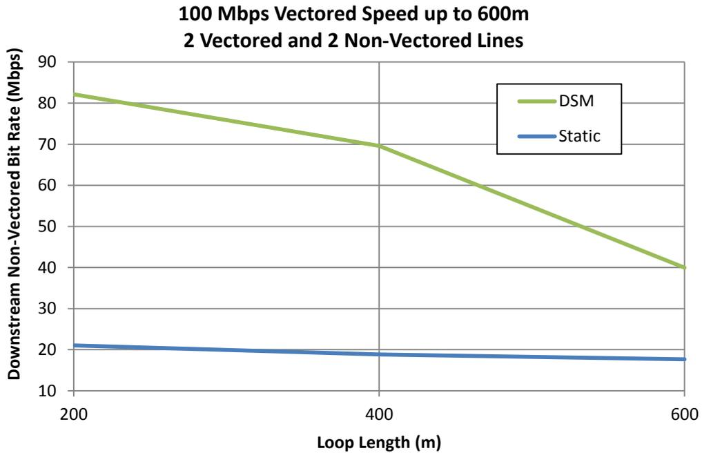
Figure 3. 2 vectored VDSL2 and 12 non-vectored VDSL2, 1% worst-case non-vectored speeds with SSM ensuring 100 Mbps on vectored lines no longer than 600 m. A 2 MHz SSM limit on non-vectored lines ensures 100 Mbps on vectored lines no longer than 600m.
