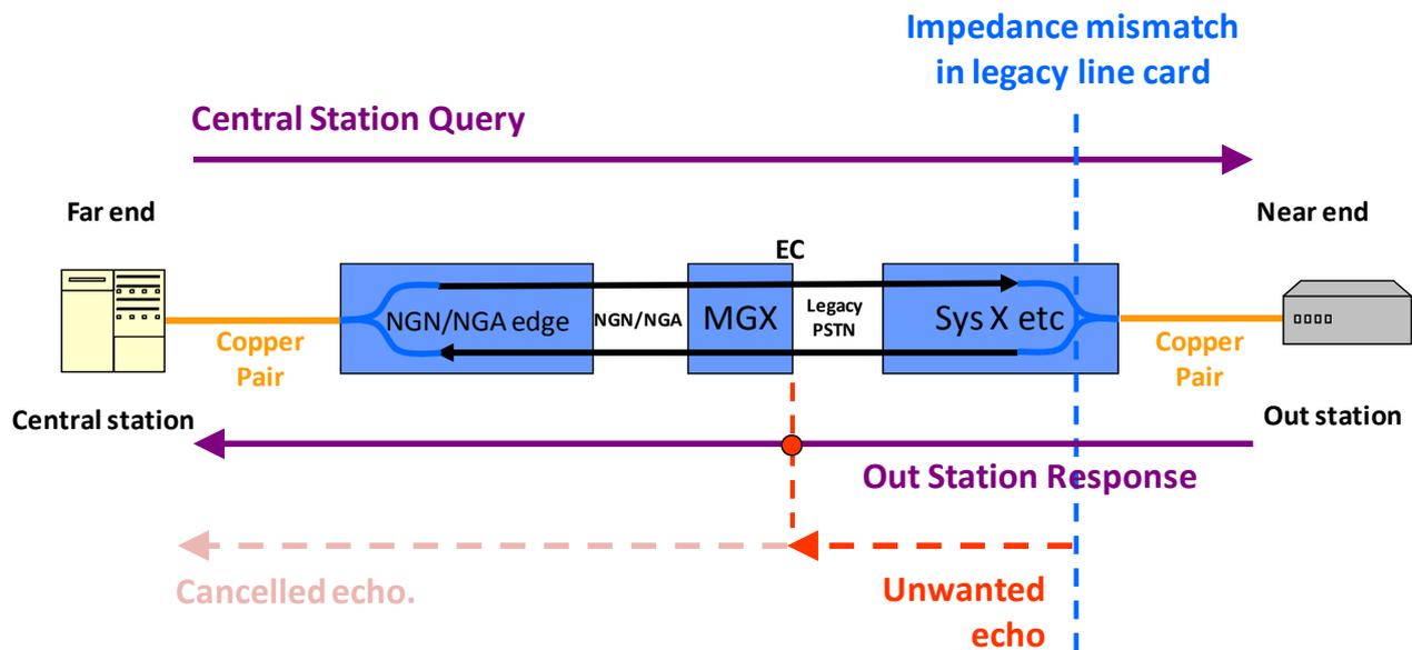
The positions of the out station and central station are now reversed from that described in Section 9.3.1. In the above diagram, the unwanted echo from the legacy line card is cancelled by the echo canceller in the Media Gateway. A fast responding out station CPE at the legacy PSTN end may have its response clipped by the NLP operation in the Media Gateway echo canceller. Only one direction of echo is shown.
