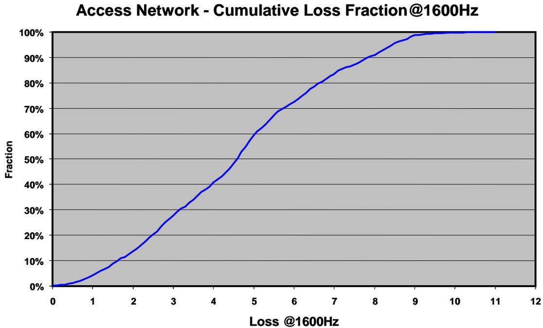
In this sample of lines, no line exceeds 15dB @ 1600Hz line loss, and 99.8% of lines are actually within 10dB @ 1600Hz line loss. However the number of lines at the extreme end of the sample is low, and these percentages cannot be guaranteed to be completely representative of the UK access network as a whole.
