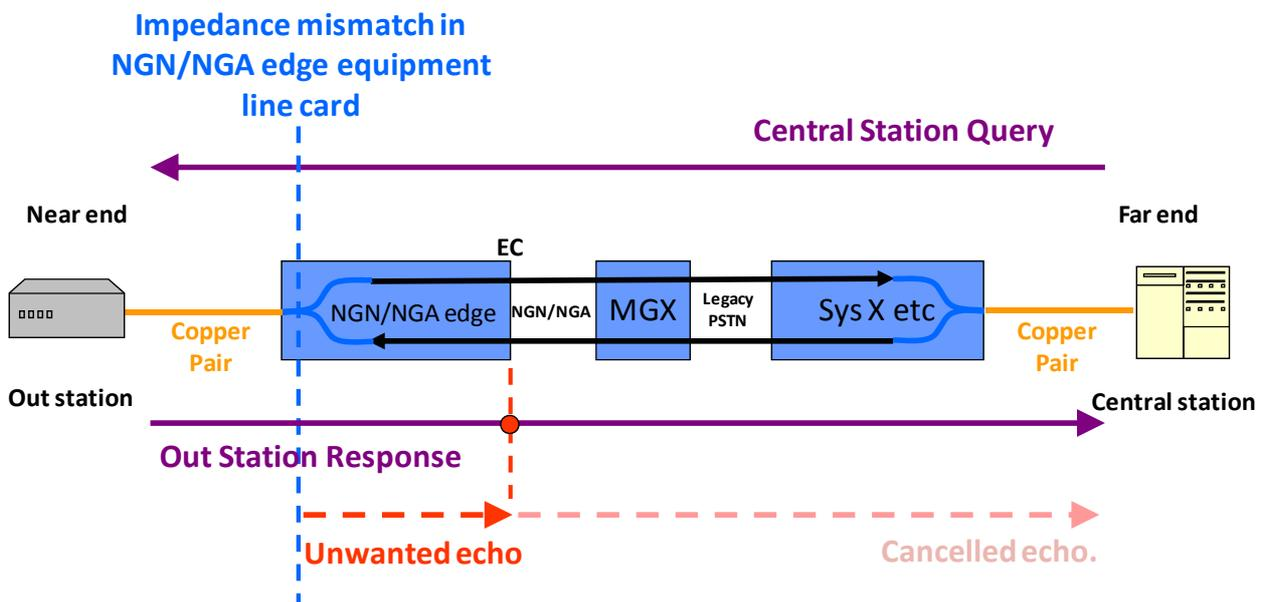
In the above diagram, the unwanted echo from the NGN/NGA edge equipment line card is cancelled by the echo canceller in that line card. A fast responding out station CPE at the NGN/NGA end may have its response clipped by the NLP operation in the MSAN / ATA echo canceller. Only one direction of echo is shown.
