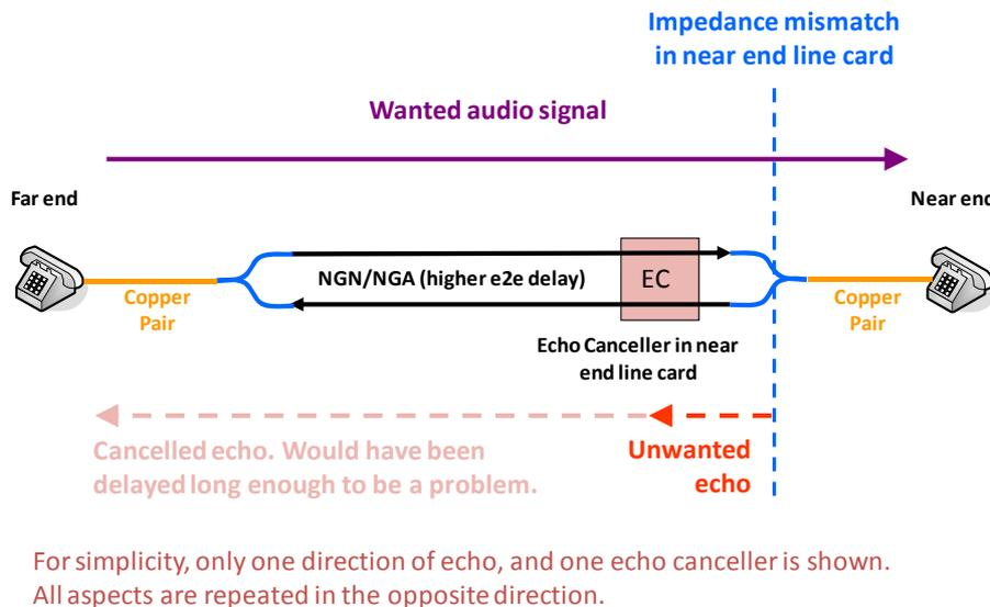
It is important to note that echo cancellers are contained in the NGN/NGA edge device (eg MSAN or ATA) but also in the Media Gateway that interconnects to TDM based legacy networks. The designs and operation of these two echo cancellers may well be different.
