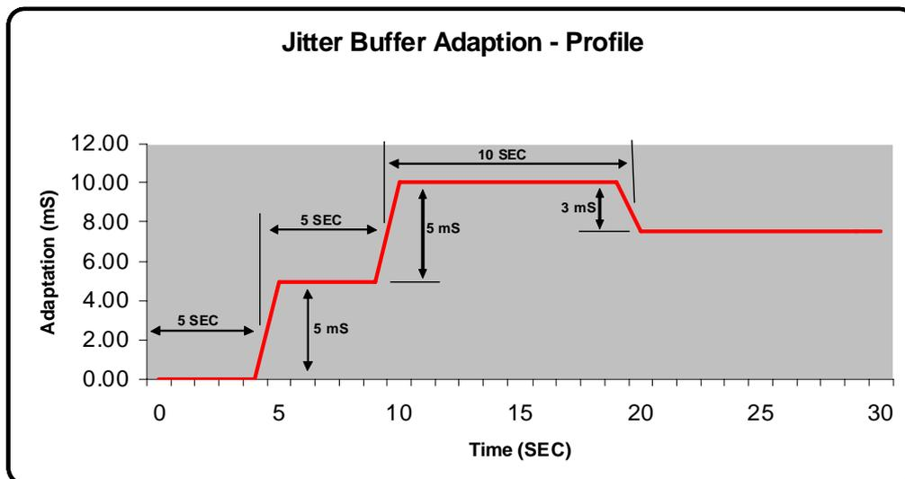
The impact of line loss on the sensitivity of VBD CPE to jitter buffer adaptations can normally be disregarded. Testing should however include relevant combinations of event/transaction reporting/polling, and other supported CPE functions, as described in Section 15.3.
