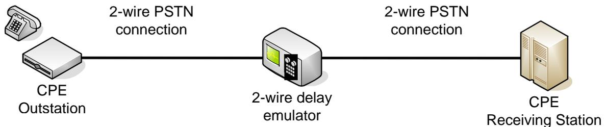
This method can be used when both ends of the VBD CPE application is available at the same location. The CPE outstation is connected to one side of the delay emulator, and dials through to the CPE central station connected to the far side of the delay emulator.
