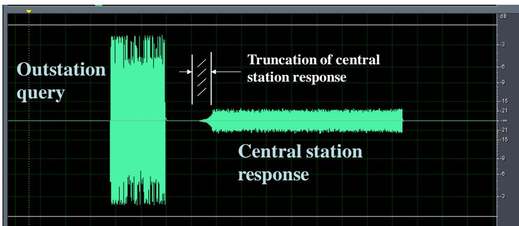
Clipping can in principle occur in two directions, as described in the next two sections.
